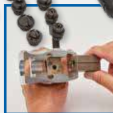
Magnetic yoke holds dies securely in place
