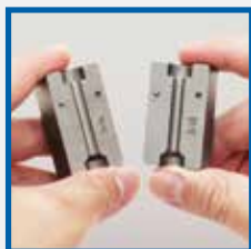
Dimples ensure accurate alignment of dies
