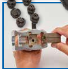
Magnetic yoke holds dies securely in place
