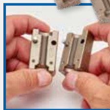
Pins ensure accurate alignment of dies
